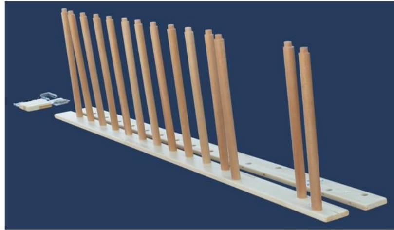
2. Fit the rungs in a side rail; align the flat side of the rung with the long dimension. Use a rubber mallet to tap the rungs in place if necessary
