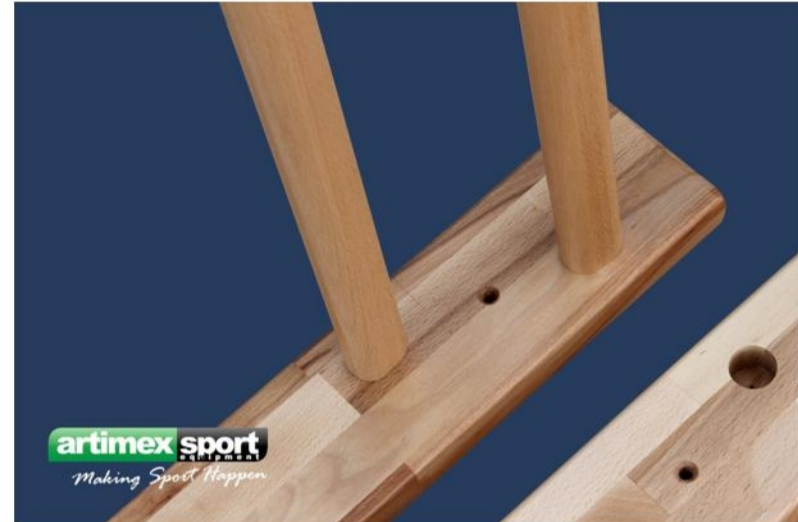
2. Fit the rungs in a side rail; align the flat side of the rung with the long dimension. Use a rubber mallet to tap the rungs in place if is necessary
